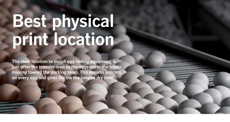
Since the eggs are cradled by the baskets, there's not a lot of room to print, so print head location and adjustment is critically important. Most printheads are installed to print on the side of the egg, producing very reliable printing and the printheads stay clean.
